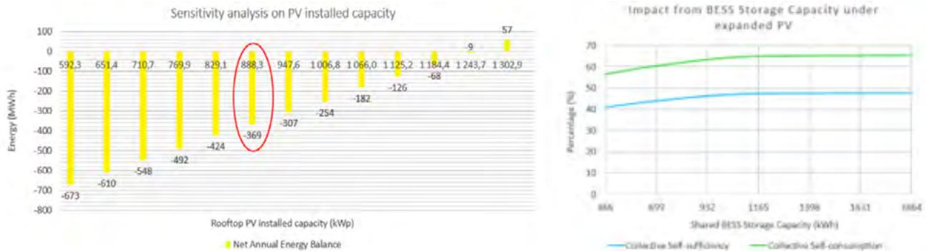
This limitation was primarily due to the restricted rated power of the BESS, constrained by the hosting company's grid connection capacity. As a result, the battery could not efficiently store the increasing PV surplus during peak generation periods. These findings suggest that locating the shared BESS within a MV grid-connected company, which typically has a higher connection capacity, could allow a more efficient BESS integration and overcoming the observed limitations.
