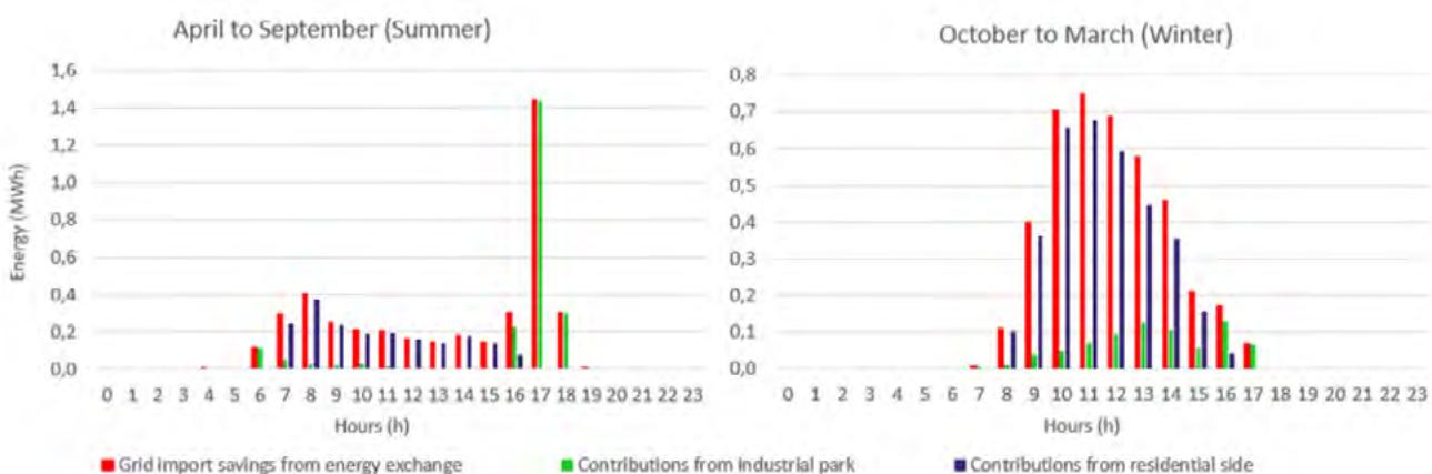
The integration of a building-level shared BESS, located within one of the low-voltage grid-connected companies, resulted in significant improvements to system performance and operational flexibility. Despite being constrained by the host site's grid connection capacity, the BESS enhanced CSC and CSS by 14% and 7%, respectively. These gains translated into an approximate 10% reduction in combined annual electricity costs for both industrial and residential users.
