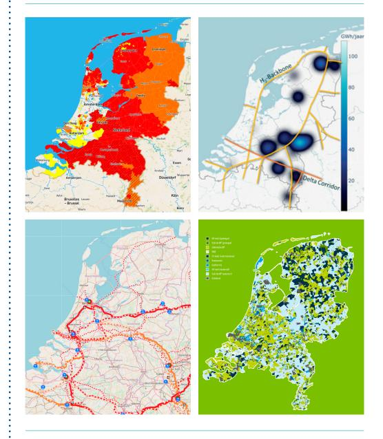
Figure 1: Four maps showing areas with relevant characteristics for decentral electrolysis. Top-left: supply-side congestion (red). Top-right: decentral industrial demand (blue) and main hydrogen infrastructures. Bottom-left: the main road (filled), water (dotted) and rail (striped) related transport & mobility corridors. Bottom-right: potential for hydrogen in the built environment (light blue).
