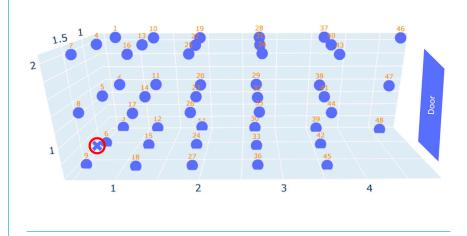
Figure 5: Side view of container showing positions of gas sensors. Red circled the gas discharge point. Gas sensor 50 is used as additional protection (with limit value of 60% of LEL).
