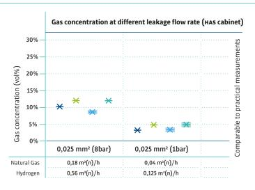
Vent: Hydrogen Vent: Natural gas Cabinet: Hydrogen Cabinet: Natural gas
