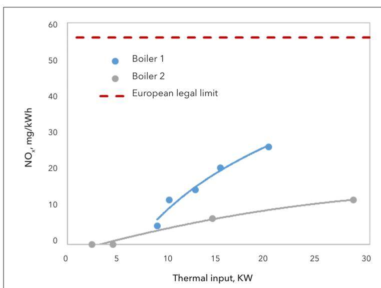
Figure 4 - Left: DNV GL/GasTerra (boiler 1) and Bekaert (boiler 2) condensing boilers in Rozenburg demonstration
