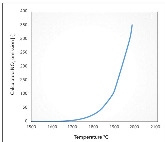
Figure 3: Calculated thermal NO formation as function temperature
